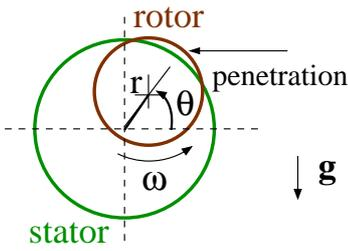
**Fig. 1.** The schema of a Jeffcott rotor with a rubbing effect, note that the stator-rotor clearance can be exceeded. We assume the restore force with a fractional power of the penetration depth.
