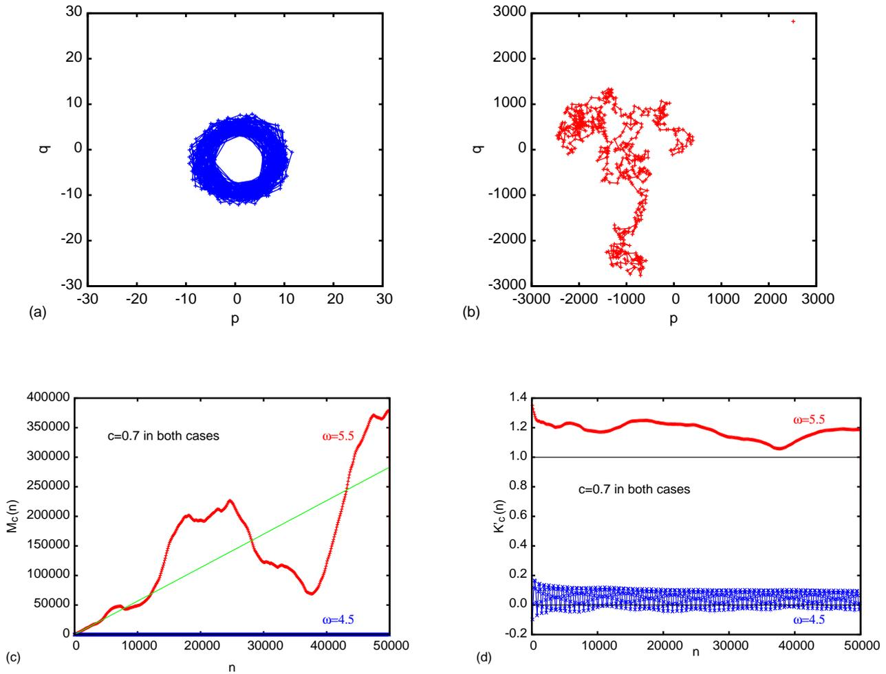
**Fig. 4.**  $p$ - $q$  phase plots for  $\omega = 4.5$  (a) and  $5.5$  (b). The length of time series was  $n_{max} = 54200$  ( $c = 0.7$ ). Note, differences in the axis scale (a,b). Total mean square displacement  $M_c(n)$  versus sampling time  $n$  for  $c = 0.7$  (c), and the corresponding parameter  $K'_c(n)$  (d). The inclined straight line (green) in Fig. 4c reflects the linear growth the total mean square displacement obtained by fitting by least squares to  $M_c(n)$ .
