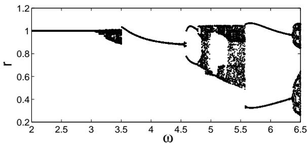
**Fig. 2.** Bifurcation diagram of the system obtained through continuation of solution during the quasistatic increase of rotational velocity  $\omega$ .
