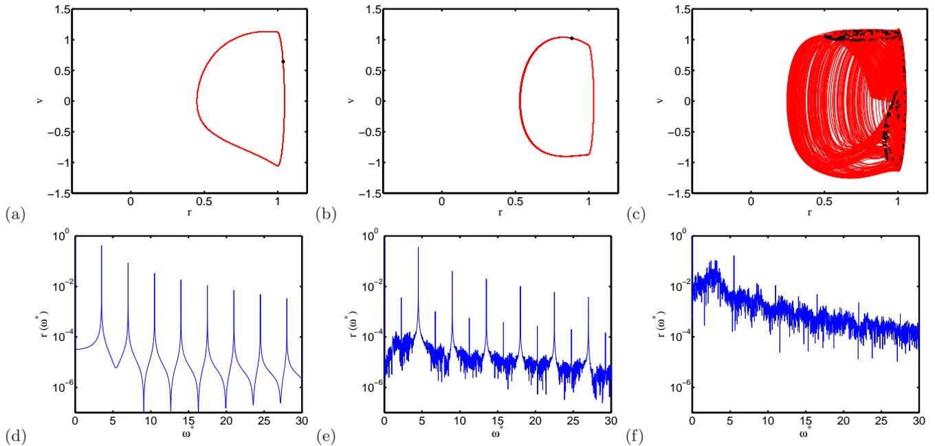
**Fig. 3.** (color online) In the upper panel – the phase portraits (with red lines) and Poincaré maps (with black points) (a)–(c) for the radial coordinate  $r$  ( $v = \dot{r}$ ); in the lower panel – the corresponding Fourier transforms  $r(\omega^*)$  (d)–(f). Rotational velocity: (a),(d)  $\omega = 3.6$ ; (b),(e)  $\omega = 4.5$ ; (c),(f)  $\omega = 5.5$ .
